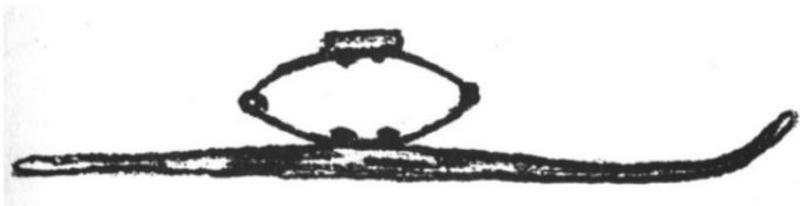
Jumper made from ash log with spring from buggy seat attached to ski.
