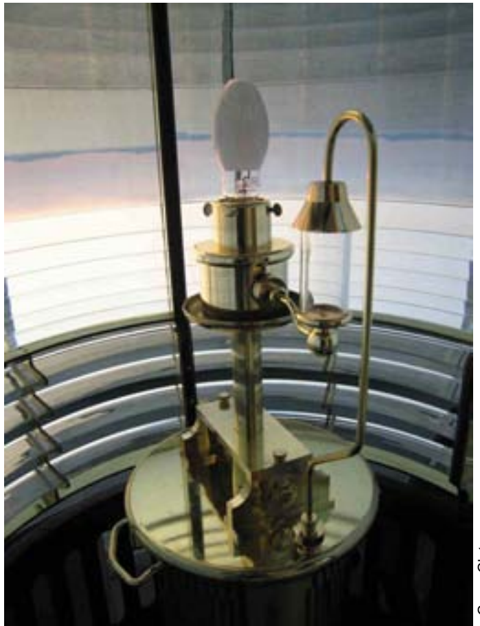
Unique lamp assembly designed by Electro-Optics of Traverse City
